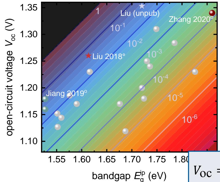
$$V_{oc} = V_{oc}^{\text{rad}} + \frac{kT}{q} \ln(Q_e^{\text{lum}})$$
