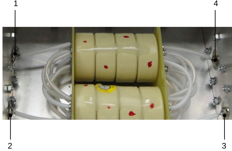
Figure 5. A photograph of the high-power 4-ports transformer. A fan is used to continuously cool down the ferrite rings and it is located on the lid of the aluminum box. The ferrite cores and the winding can be clearly distinguished. 1: port (1); 2: port (2); 3: port (3); 4: port (4). Coaxial cables (i.e., with inner and outer conductors) are used as winding wires. A closer look at port-1 shows the mounting of the coaxial winding to a ‘7/16’ connector. The ports of the transformer are marked in figure 1.
