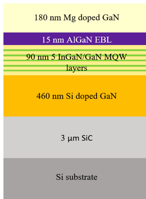
FIG. 2. A schematic diagram of the sample structure.
