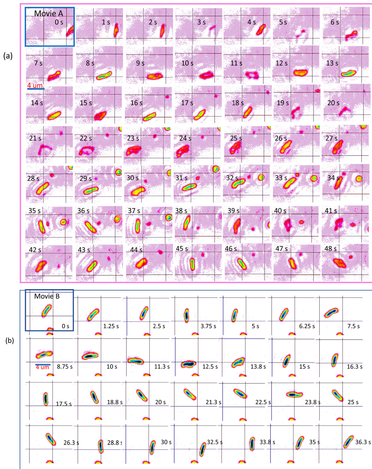
Fig. 4. The “enhanced” phase contrasted images for the orientations and rotations of a GO-sheet at a (a) low-frequency (of 100 Hz) and (b) a high-frequency (10 kHz) controlled spatial-temporal images and its corresponding data movies are shown Movie A and Movie B, respectively. The field amplitude for both frequencies is as 10 V/mm, under AC sinusoidal waveform.
