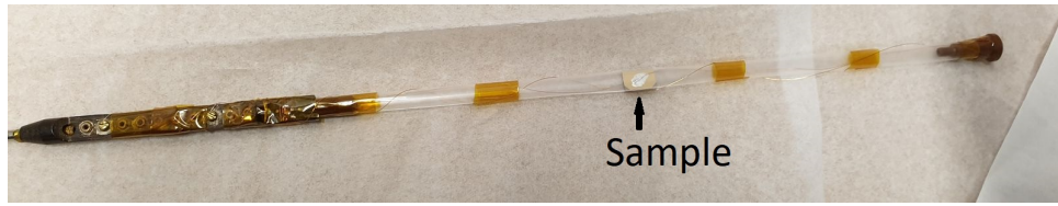
Figure 3.10: Picture of a sample mounted in the MPMS magneto-electric option.
