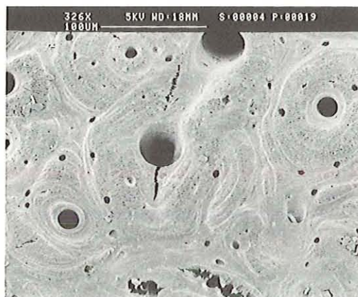
Fig. III.27. Cracks in HCl-etched CPD-specimens (SEM: BSE-mode) a) cracks with fibrils, b) cracks without fibrils
