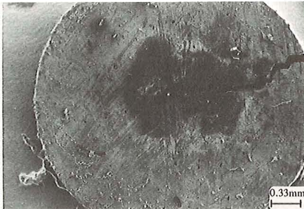
Fig.III.32. Damage in dimpled TEM-specimen
