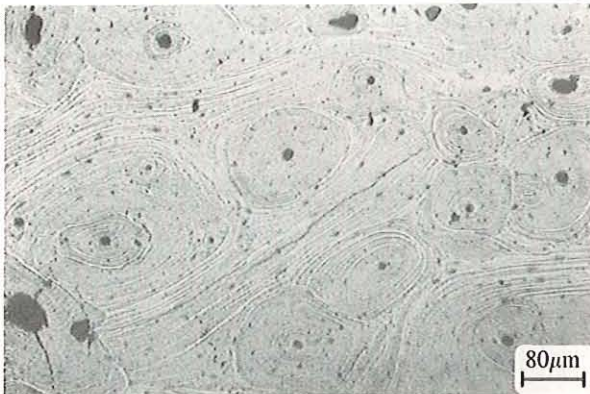
Fig. III.25. State of goat bone specimens after polishing and before drying a) radial cracks through Haversian systems, b) cracks following the lamellae
