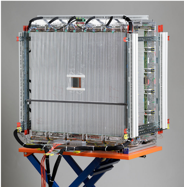
Fig. 2 The STS1 prepared for installation in HADES. (Photo: courtesy of Forschungszentrum Jülich GmbH.)
