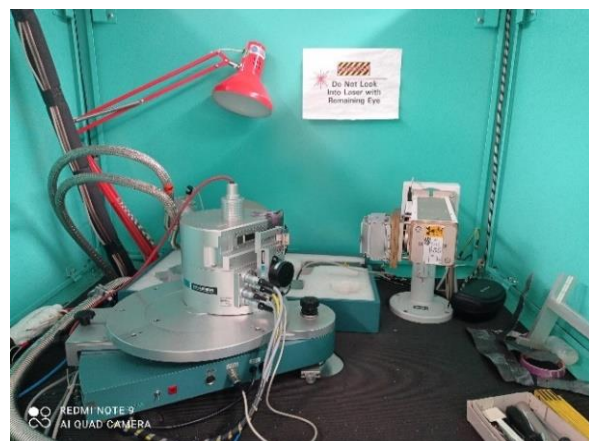
Fig.4.3 ( left) Schematic view of the G670 diffractometer [8], (right) Huber G670 Powder Diffractometer at JCNS-2.
