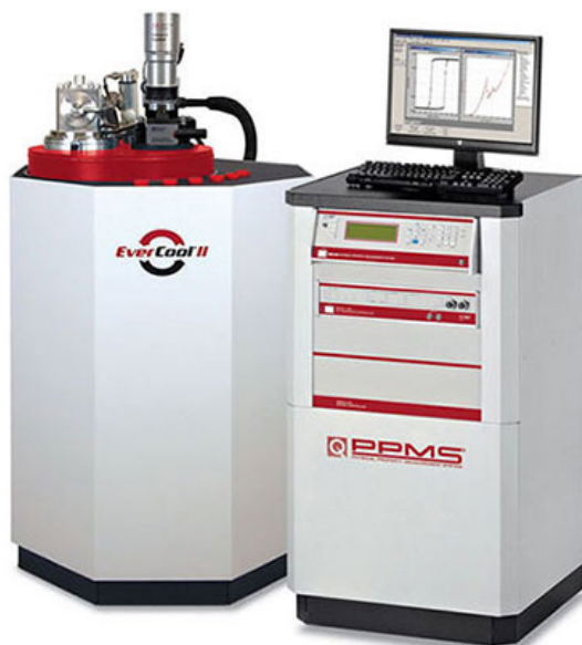
Figure 3.9: Picture of quantum design PPMS system. Source: www.qdusa.com/products/ppms.html
