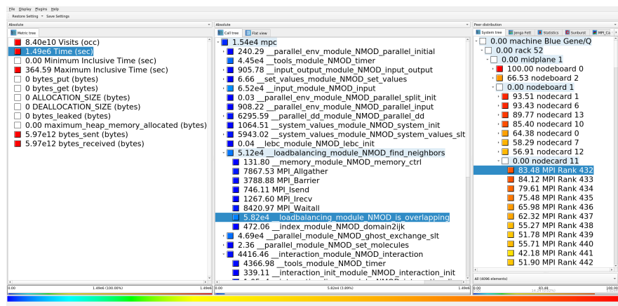
Fig. 3: MP2C measurement example with 4096 processes on a Blue Gene/Q highlighting the limited global overview with the default system-tree due to the limited number of locations shown at the same time.
