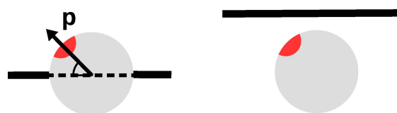
Figure 1. Cartoon of an active colloid trapped at (left) or close to (right) a fluid interface (black solid line). The red spot represents the area in which the catalytic reaction takes place.
