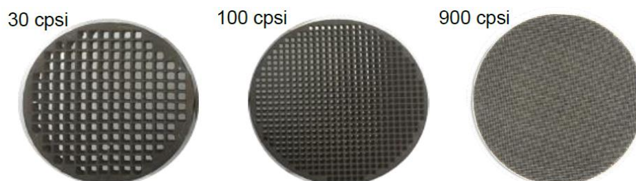
Figure 4. Catalyst specimen with different cell densities
