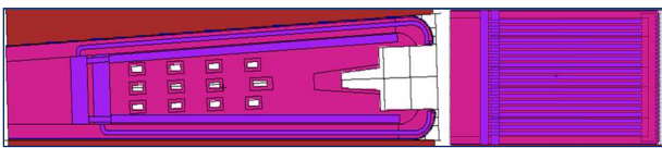
Figure 7: Toroidal (left) and poloidal (right) planes of the MCNP model of the DSC.
