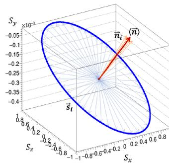
Figure 1: Spin tracking simulations using the reference particle moving on the closed orbit. The invariant spin axis is the vector perpendicular to the plane that is defined by the spin wheel. For each turn  $i$ , the normal vector  $\vec{n}_i$  is calculated. The average normal vector  $\langle \vec{n} \rangle$  is then considered as the invariant spin axis.
