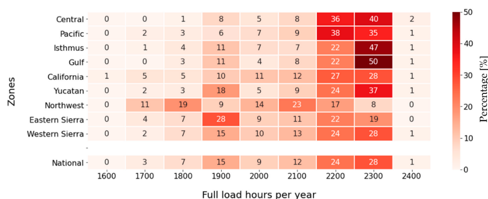
Figure 8. PV full load hours by zone.
