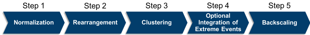
Figure 2. Time series clustering procedure for energy system models.
