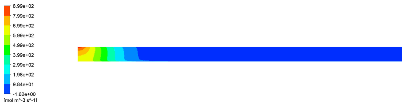
Fig. 6. Reaction kinetics of the independent RWGS, T = 900 °C, p_t = 30 bar, \text{H}_2:\text{CO}_2 = 1:1 , and \text{GHSV} = 900 \text{h}^{-1} .
