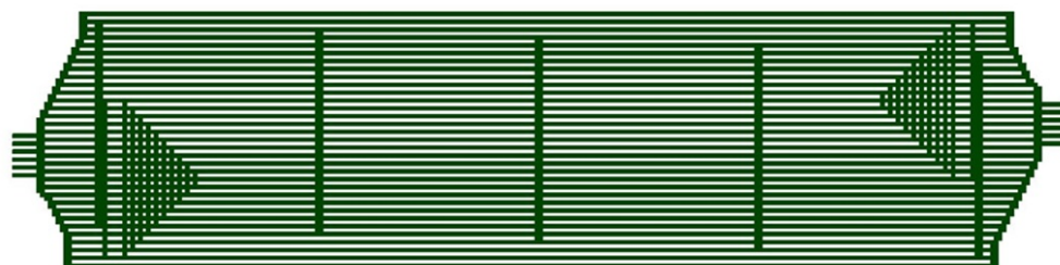
Figure 15. Simplified model of the coolant flow field with added manifold regions.
