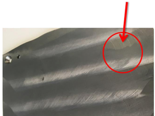
Figure 13. ODS steel plate after removing the capsule residues and preparation of the surface for diffusion bonding. The arrow indicates one of several areas of grooves (chatter marks) that occurred due to vibrations during milling, which were used as a robustness test for the plating process.
