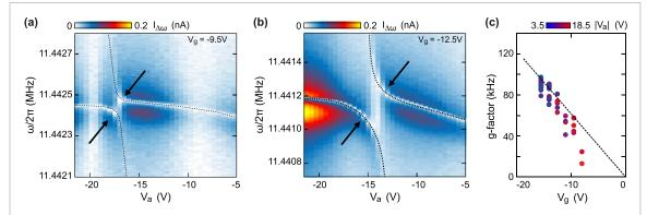
**Figure 4.** (a), (b) Zoom of avoided crossings. The g-factor is proportional to the minimal distance between the resonance lines (dashed black lines). (c) The g-factor extracted from the avoided crossings as a function of  $V_g$  reveals a tunable mode coupling. The dashed black line is the g-factor arising from the electrostatic force.
