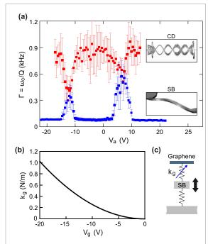
**Figure 5.** (a) Linewidths  $\Gamma=\omega_0/Q$  of the interacting modes at  $V_{\rm g}=-14$  V. The linewidths of the two modes (see insets and supplementary figure 5) become equal near the avoided crossing. (b) The tunable electrostatic softening spring  $k_{\rm g}$  as a function of  $V_{\rm g}$ . (c) Schematic illustration showing how  $k_{\rm g}$  connects the graphene membrane (coupled to the MEMS actuator) to the suspended silicon beam.
