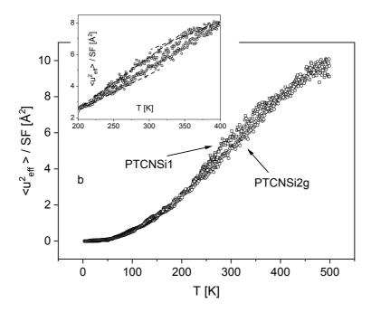
Figure 3b: Effective mean squared displacement  $< u^2_{eff} > versus temperature normalized by the scaling factor SF described in the text: squares – PTCNSi1, circles – PTCNSi2g. The inset enlarges the data in the temperature range from 200 K and 400 K. Lines are guides for the eyes.$
