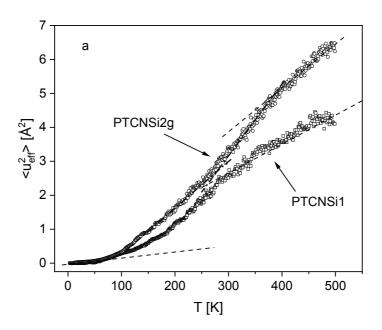
Figure 3a: Effective mean squared displacement  $< u^2_{eff} > versus temperature: squares - PTCNSi1, circles - PTCNSi2g. Lines are guides for the eyes.$
