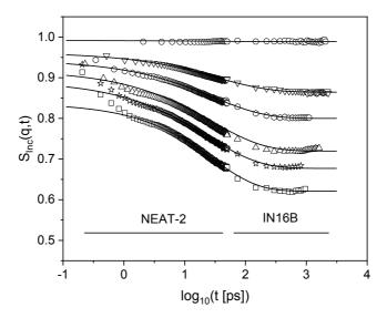
Figure 4. Incoherent intermediated scattering function  $S_{Inc}(q,t)$  versus time for PTCNSi1 for different q vectors at 150 K: circles  $-0.3 \text{ Å}^{-1}$ , down sided triangles  $-0.84 \text{ Å}^{-1}$ , octagons  $-1.13 \text{ Å}^{-1}$ , triangles  $-1.4 \text{ Å}^{-1}$ , asterisk  $-1.61 \text{ Å}^{-1}$  and squares  $-1.78 \text{ Å}^{-1}$ . Lines are fits of equ. 3 to the corresponding data.
