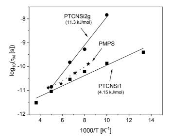
Figure 7. Relaxation time for the methyl group rotation versus inverse temperature: Squares – PTCNSi1, circles – PTCNSi2g and asterisk – poly(methyl phenyl siloxane) (PMPS). The data for PMPS was taken from ref. 32. Lines are fits of the Arrhenius equation to the corresponding data.
