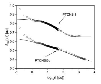
Figure 6. Comparison of the incoherent intermediate scattering function  $S_{Inc}(q,t)$  versus time for PTCNSi1 (squares) and PTCNSi2g (circles) at q=1.78 Å<sup>-1</sup> and T=125 K. Lines are fits of equ. 3 to the corresponding data. The data are shifted along the y-scale for sake of clarity.
