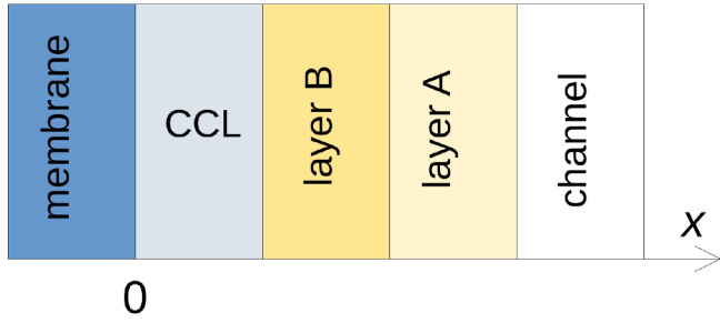
Fig. 1. Schematic of a PEMFC cathode with the GDL (layer A) and MPL (layer B).
