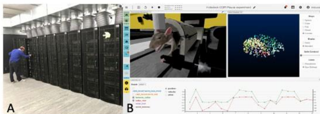
Fig. 5 Technologies driven by neuroscience. A The million-processor SpiNNaker machine at Manchester. B The user interface of the Neurorobotics Platform NRP, executing the virtualized copy of a real mouse experiment. The mouse body shown in the live rendering on the left is connected to a brain simulation that controls its muscle activations. Body movements are plotted in the graph at the bottom.
