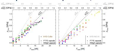
To assess the reproducibility of the cell loading, multiple tests with both M1D variants and two capsule materials (PTFE, AlMg5) are performed.
