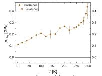
The pressure drop at low temperatures is determined by cooling down a cell loaded to 0.45 GPa.
