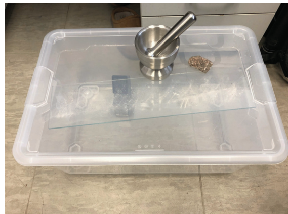
Fig. 7: Experimental set-up. Granite powder is produced in a mortar and deposited on a glass plate located in a closed box. The glass plate is cleaned with soap water, acetone and isopropanol. The humidity in the closed box is changed by including in the box a cup of water or humidity absorbing salt. The glass plate with granite powder is kept in the box for 24 hours to obtain thermal (kinetic) equilibrium between the water molecules at the interface and in the gas phase.
