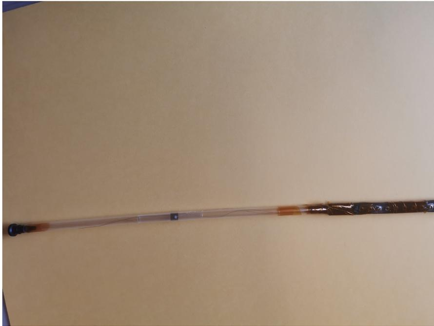
**Figure 3.8:** Sample connected with SQUID holder by copper wire
