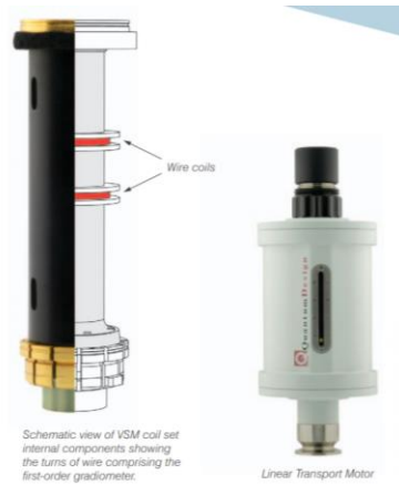
Figure 3.7 VSM coil set and linear transporter (figure taken from ref. 25 )
