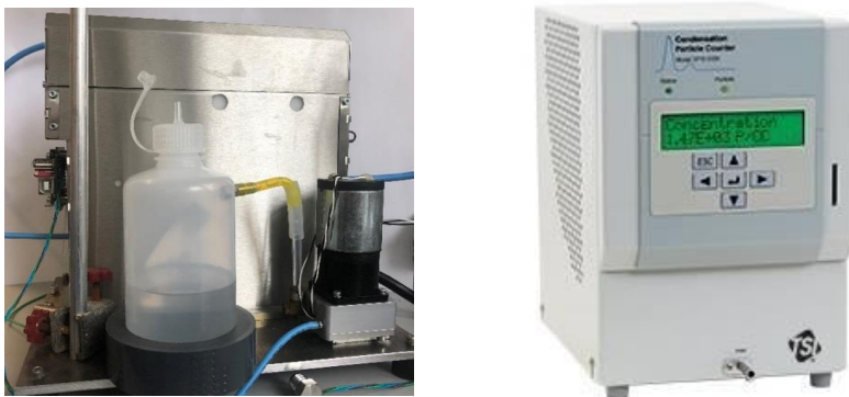
Fig. 25: Picture of the two current CPC models used in the experiment: Sky-CPC 5.411 (Grimm) on the left and CPC 3772-CEN on the right (Photograph © TSI Inc.).
