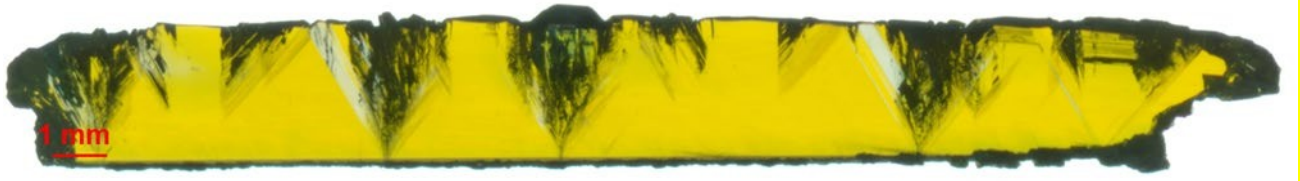
Fig. 4 Cross sectional view of a 3 mm thick free standing 3C-SiC boule. Even in the case of a low density, the expansion of the protrusion defects during growth (bottom = early growth stage, top = final crystal surface) leads to an almost complete spreading of the distorted crystal at the crystal end.
