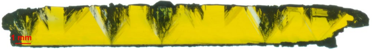
Fig. 4 Cross sectional view of a 3 mm thick free standing 3C-SiC boule. Even in the case of a low density, the expansion of the protrusion defects during growth (bottom = early growth stage, top = final crystal surface) leads to an almost complete spreading of the distorted crystal at the crystal end.
