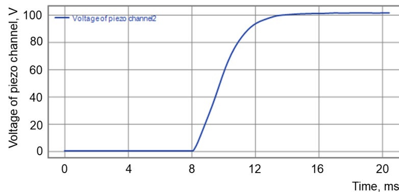
Figure 8. Time characteristics of the piezo element P-602 [36] used for the fast opening valve.
