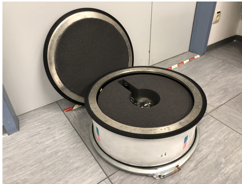
Figure 5. Magnetic transport box [18] with a single glass ball for polarized ^3\text{He} gas. Alternatively, boxes are available that can accommodate three glass balls at the same time.
