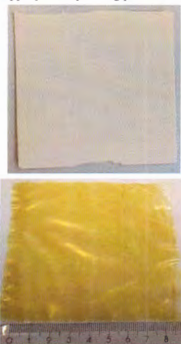
Figure 1. Ceramic diaphragm prepared by thermal spray coating (left) and LDH-based membrane (right).
