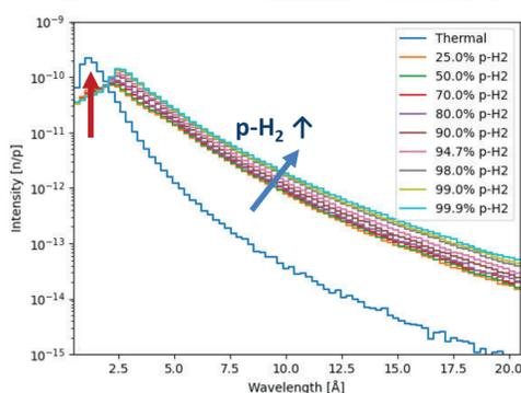
→ Decreasing intensity with increasing amount of orthohydrogen due to higher scattering cross section
