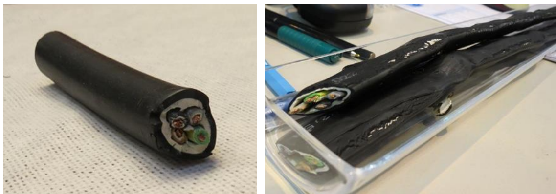
Figure 6: Flame retardant non-corrosive (FRNC) power cable sample (left), pressed cable sample (right)
