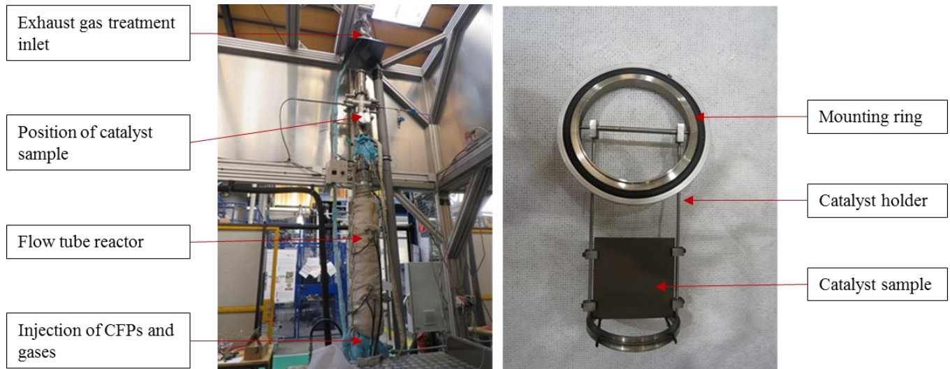
Figure 3: Vertical reaction tube (left), catalyst holder with sample (right)
