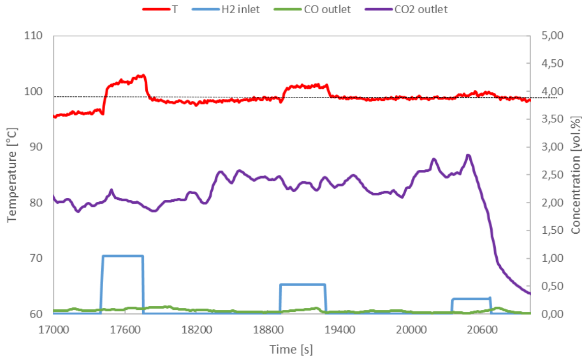
Figure 11: Pd catalyst behavior during well-ventilated combustion (RF-B-01)
