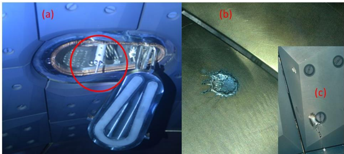
Figure 8. View of the magnetic flux surface measurement probe installed on the upper side in module-1, (a) shows the probe with shutter opened, the melted steel drops are on the panel below (b) and neighboring graphite tile (c).
