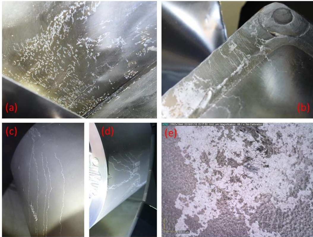
Figure 7. Arc traces observed on the front side (a) and backside (b) of a panel, ports (c) & (d) and an enlarged view of a random arc trace with microscope (e).
