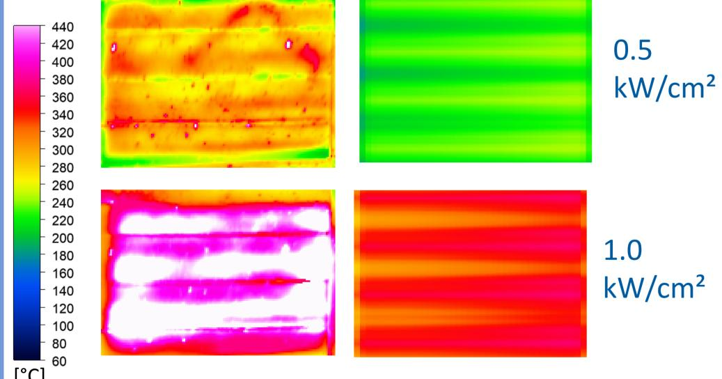
CFD simulation IR measurement
