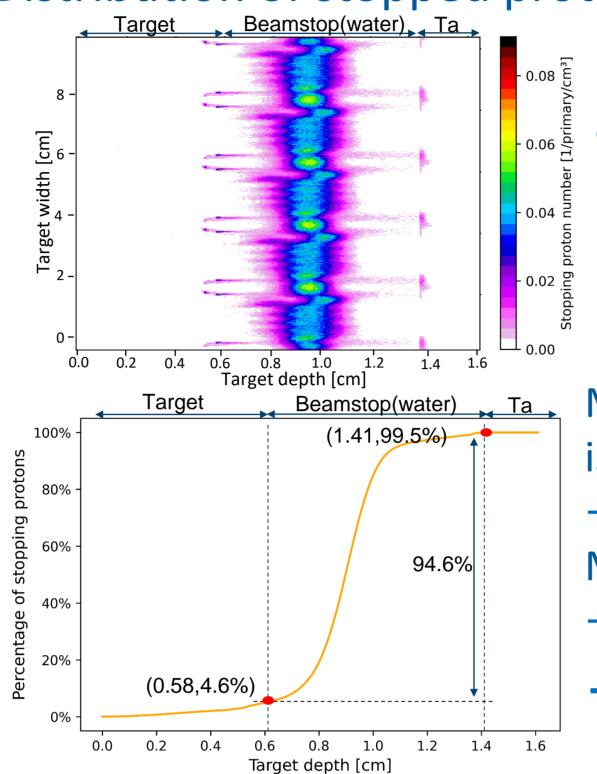
Only 4.6% of protons stop in the target, 93.2% accumulate in the beamstop (water).
