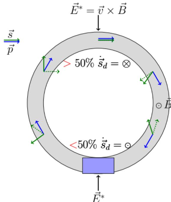
$E^*$  field in the particle rest frame tilts spin due to EDM up and down  $\Rightarrow$  **no net EDM effect**
