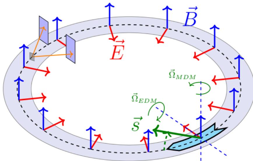
$$\frac{d\vec{s}}{dt} \propto \underbrace{d(\vec{E} + \vec{v} \times \vec{B}) \times \vec{s}}_{= \vec{\Omega}_{EDM}}$$
