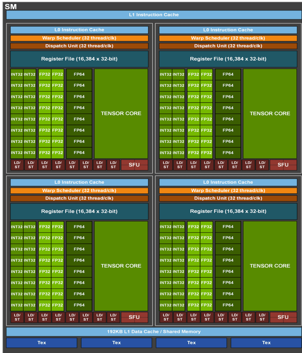
Figure C.7.: The figure depicts the design of a Streaming Multiprocessor (SM) in the Ampere architecture used by the A100 GPU [54].
