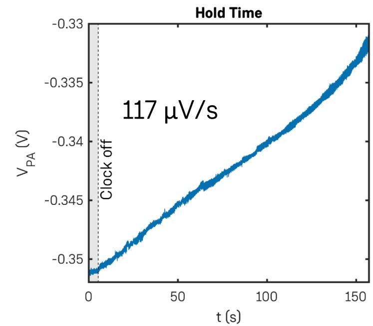
Fully Autonomous DC Bias-DAC Operating at 45mK
