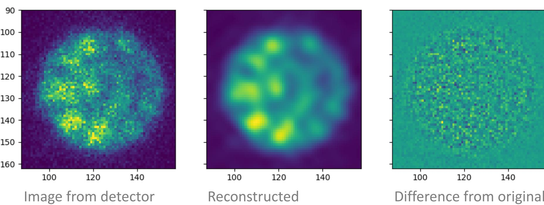
Represent detector frame in  $16 \times 16$  HO-basis
