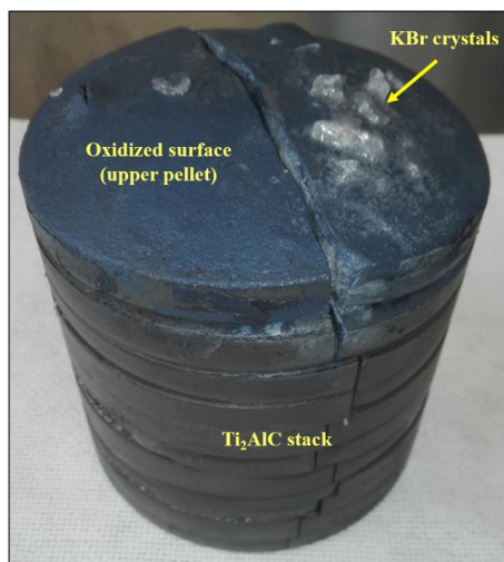
Figure 3. 1: Stack of 10 \text{Ti}_2\text{AlC} pellets ( \varnothing 100 mm) retrieved after \text{MS}^3 . Each pellet is ~15 mm thick.
