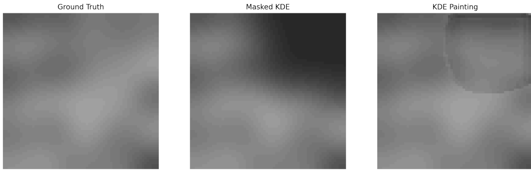
Figure 32: A training example from the Density Inpainting model. The masked KDE is the result of computing a KDE on an image of segmented cell locations, where the cells within the masked area have already been removed. The KDE painting is a composition of pixels from the model's output and the ground truth image, not the masked KDE. This painting is for evaluation purposes only, since only the masked area has to be sampled from during inference.
