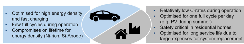
Figure 5. Requirements for EVs and stationary storage systems
